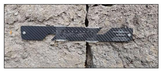
The G1.5 crack monitor is a precision instrument designed to monitor and track the evolution of crack openings. It stands out due to its **carbon construction** and a **high resolution of 0.02 mm**.
