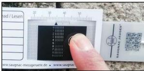
The G1+ gauge is recommended for monitoring the gap between parallel-lipped cracks. It provides reliable measurements with 0.05 mm resolution.
