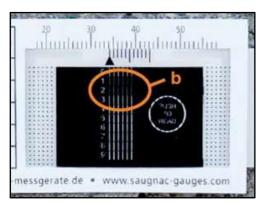
The mark ▲ on the vernier is located between 34 and
