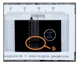
The mark A on the vernier is located between 34 and 35
