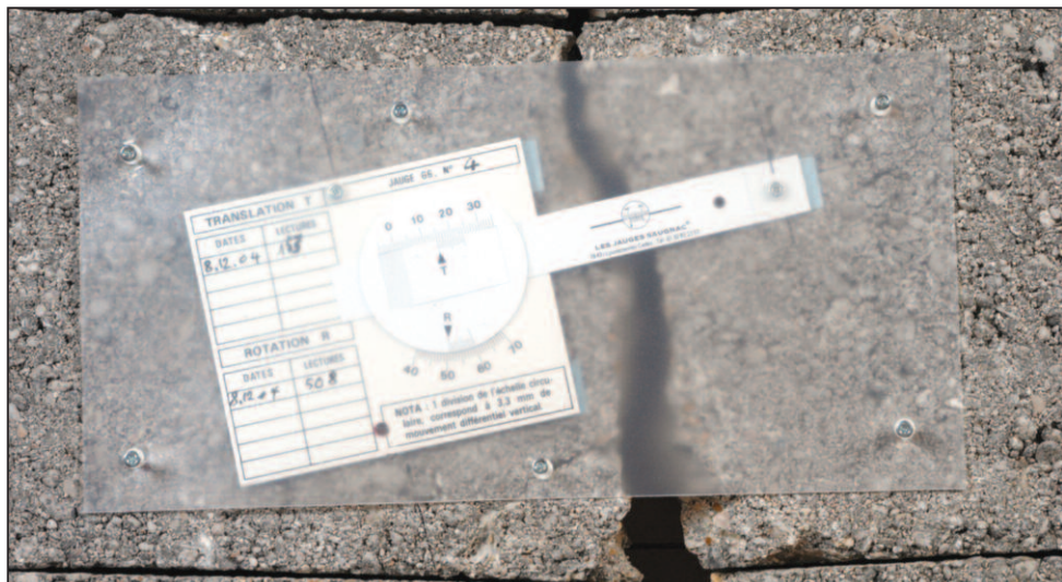
Fixing the G6 gauge and its protective cover with plugs and screws
