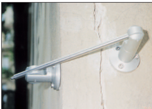
Analysing the changes in cracking arising in panneling within the framework plane.
