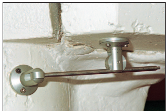
Analysing the evolution of a compression joint
