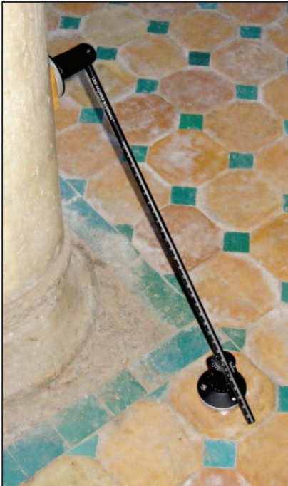
Example of installation of the 3Dim. gauge with extension. The baseplate of the post (B1) is attached onto the column by means of a wooden mount which has one concave surface.
