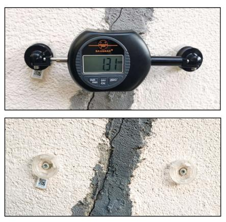
The E1 gauge is recommended for monitoring cracks on 1 axis (gap) or 2 axes (gap + shear).
