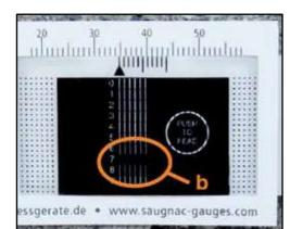
The mark 🔺 on the vernier is located between 34 and 35
