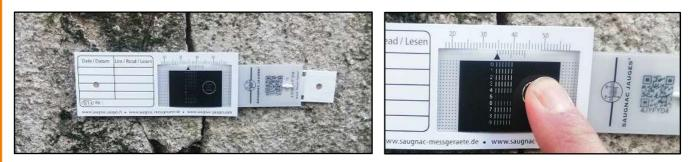
The G1+ gauge is recommended for monitoring the gap between parallel-lipped cracks. It provides reliable measurements with 0.05 mm resolution.
