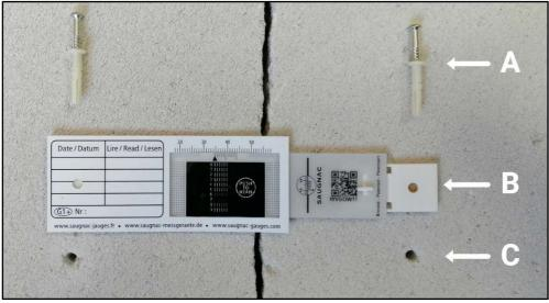
A: Impact anchors B: Hole ø4 in the strip C: Hole ø4 in bracket
