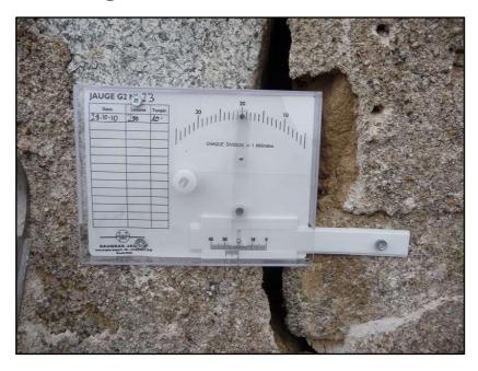
The G2 Gauge is a precision instrument designed to measure and record variations in the spacing of cracks or expansion joints located in the same plane. It offers a resolution of 0.1 mm, allowing precise monitoring of structural movements.
