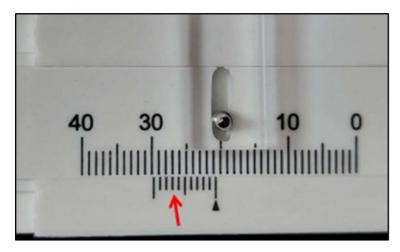
Read according to the vernier principle:
