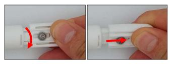
4. Fix the gauge to the crack using the screws supplied
