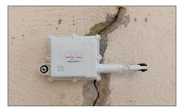
The R1 gauge is a remote crackmeter with 3 measurement sensors:
